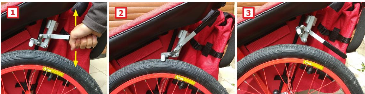
Figure 28 1 – grip additional parking brake 2 – brake is fully engaged 3 – brake is released
